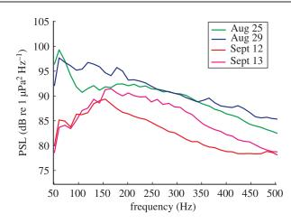
Figure 2. Power spectrum density level (PSL) of background noise in the range 50–500 Hz from 2 days before (25 and 29 August 2011) and 2 days after 11 September 2001 (12 and 13 September 2011) with identical sea-state conditions. Overall noise levels (PSL in dB re 1  $\mu$ Pa<sup>2</sup> Hz<sup>-1</sup> are lower and the peak frequency (Hz) of the noise shifted to a higher frequency post-9/11.
